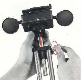
2) Pull out the rear plate of the PS-4 by the indent on the left side and connect it to the front rim of the lens in use by pressing the snap-on buttons on the top and bottom of the rear plate
